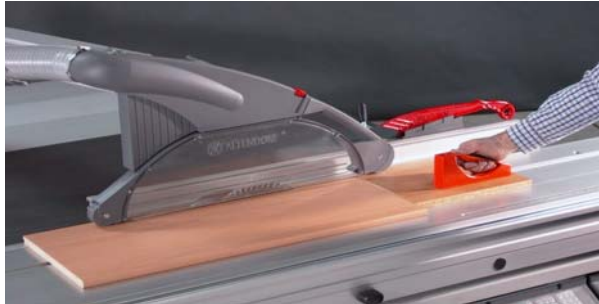
Fig. 3-9: Cutting of strips
