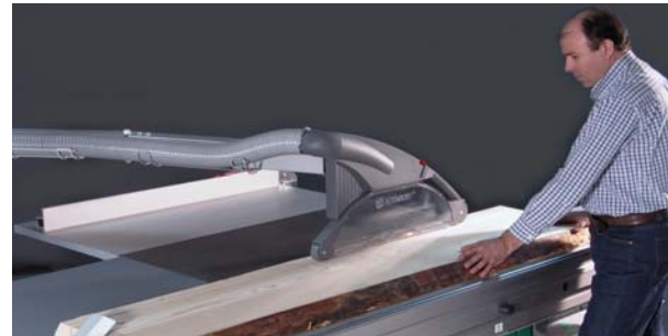
Fig. 3-7: Edge cutting (trimming)
