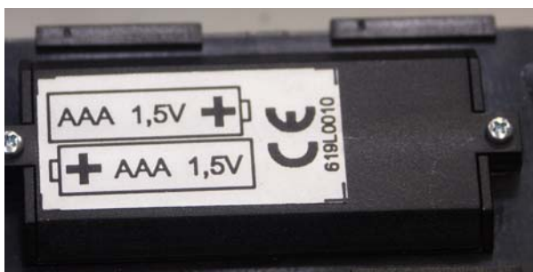
Fig. 7-11: Loosen and withdraw screws and remove cover
