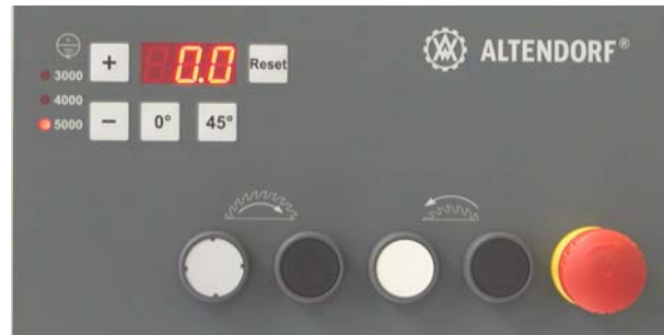
Fig. 7-5: Operating panel on eye level
