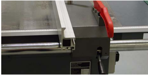
Fig. 3-5: Flat position of the extension fence
